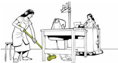
5. The operator uses the magnetic brush under the table to check for needle fragments.
