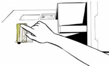
The needle dispensing person inserts the pieces of broken needle through the opening into the collection container.
